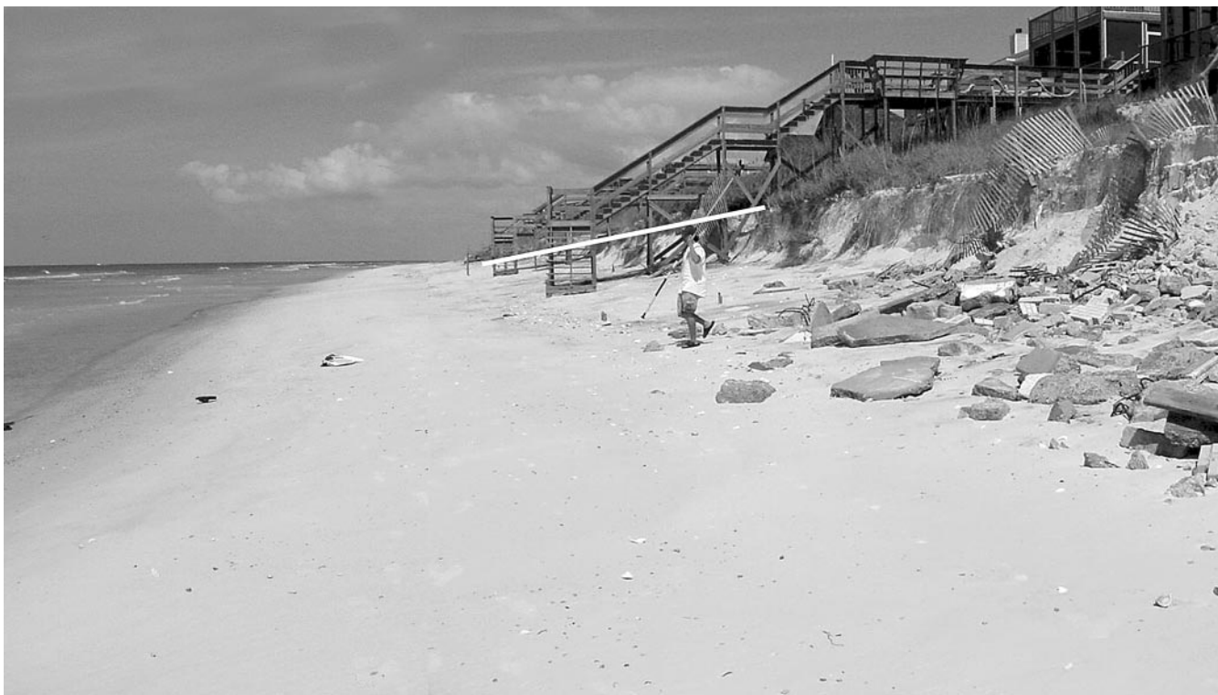
Figure 7. Study site S6_SJ2 at St. Joseph Peninsula looking north. The white line shows the prestorm dune level at the dune walkover (indicated by the different color of the wood). Photo was taken on September 23, 2004, a week after the Ivan impact.
