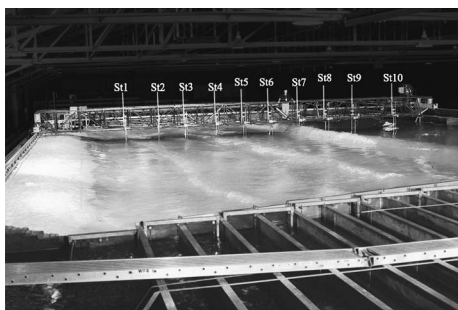
Figure 1. The LSTF during a plunging wave run, showing the instrument bridge (top) carrying current meters and wave gauges. Channels at the bottom of the photo are sediment traps to measure the sediment transport rate. The generated wave conditions are comparable to average conditions along many low-wave-energy coasts.
