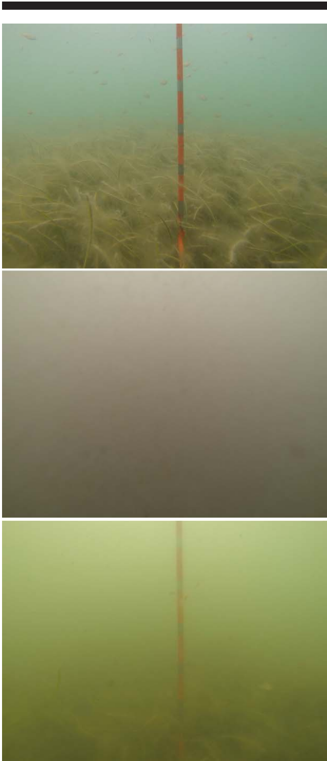
Figure 4. Underwater photos of turbidity increase and decrease during the dredging operation. Upper: Condition before the dredging operation; the dense seagrass extends about 20 cm from the seabed. Middle: Condition at the peak of the dredge turbidity plume; the reference rod about 0.5 m in front of the camera has become invisible. Lower: Condition 50 minutes after the turbidity peak; the visibility has recovered considerably. (Color for this figure is available in the online version of this paper.)
