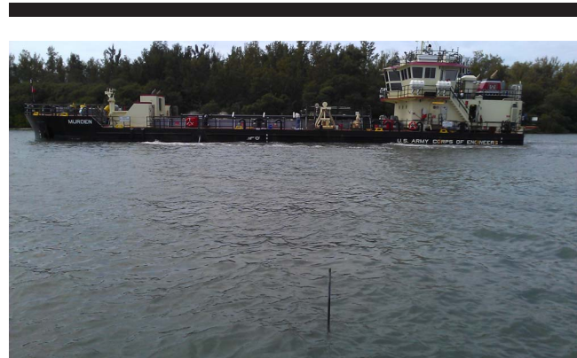
Figure 2. The USACE special operations hopper dredge, Murden, passing in front of the measurement site (metal pole at the bottom of the picture). The slurry was pumped into the container of the dredge. The overflow is visible along the side of the vessel. (Color for this figure is available in the online version of this paper.)
