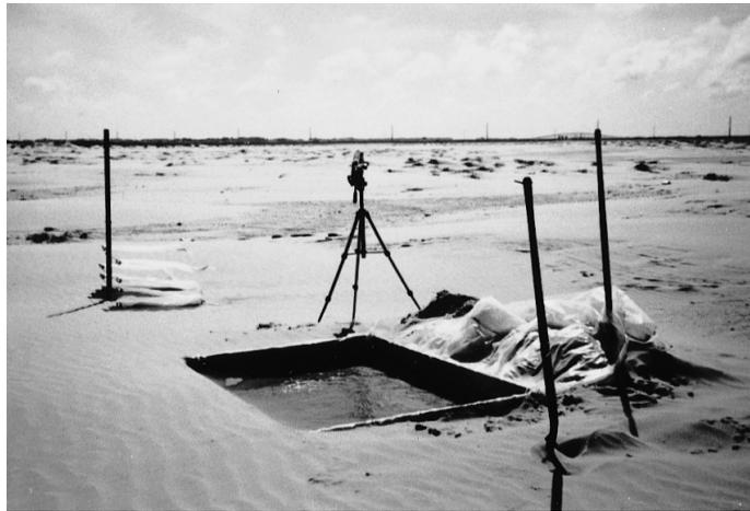
Figure 2. Field deployment of the water trap on Padre Island, Texas. Sand is blowing from south to north (left to right), as can be seen from scour around the shovel in the right foreground and the full extension of sieve-cloth bags of a vertical trap in the left background
