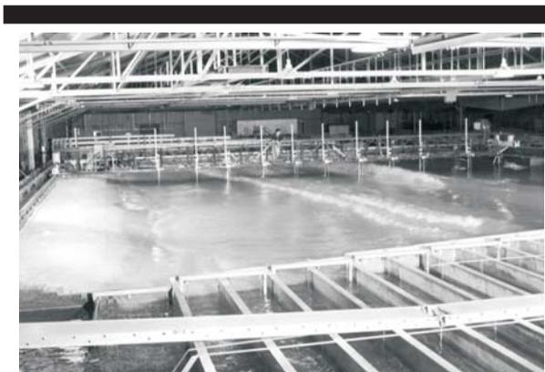
Figure 1. The LSTF during a plunging-wave case, showing the flow channels (bottom) and the instrument bridge (top) carrying the locations of the FOBS sensors (vertical bars). The locations of the FOBS sensors (vertical bars) are identified by referring the
