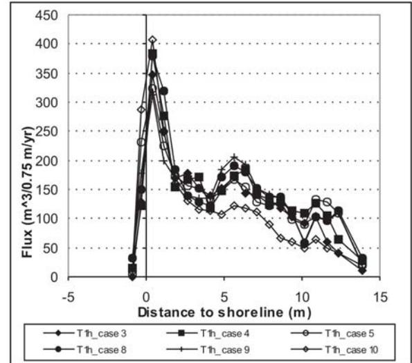
Figure 6. Repeatability of cross-shore distribution of longshore sand transport.
