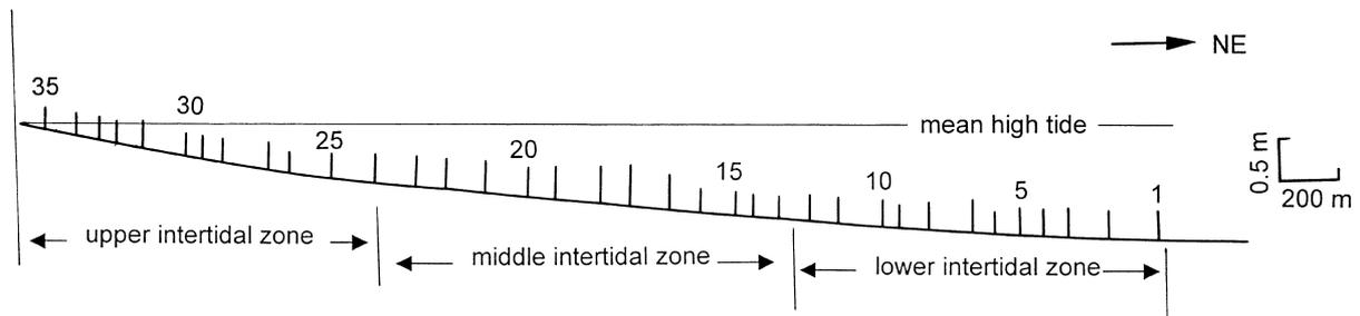
Fig. 2. Tidal-flat profile at Donghai Farm on the southern flank of the Yangtze delta, and locations of the 35 elevation rods. Every fifth elevation rod is labelled.
